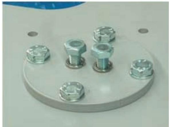
*PLACE BLADE SUPPORT WITH DISC OVER THE SHAFT AND CLAMP SCREWS
